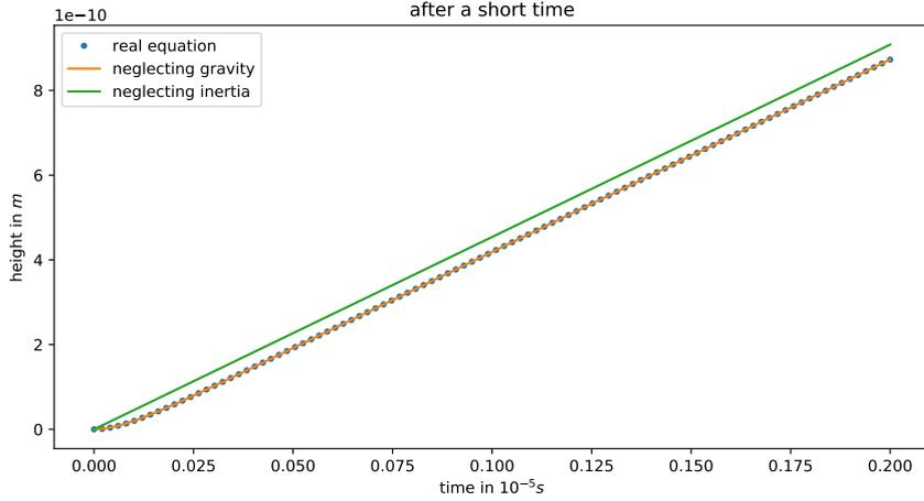
Figure 2: Numerical comparison between solution to (W) and simplified version for vessels in a short time ( $C = 1000$ )
